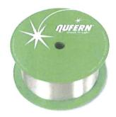
Nufern's broad line of PM fibers now includes PM1060L & PM1060L-FA fibers. These fibers are optimized for operation at 1060 nm and feature a low 0.085 NA (L). They are ideally designed for pump combiner and coupler applications for singlemode fiber lasers. The PM1060L fiber is a single clad fiber and PM106-FA is double clad fiber to cover all your application needs. Utilizing the PANDA design, these fibers demonstrate superior polarization control, resulting in increased system
